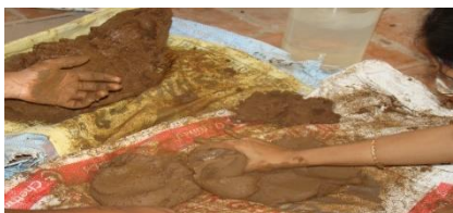
Fig.1. Mixing of brick materials
