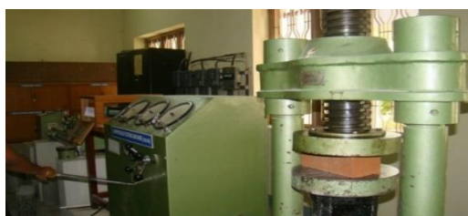
Fig.3. Compression testing of the specimen
